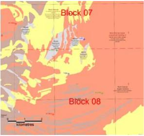
Sample of seabed texture sheet derived from backscatter and bathymetry data (UKHO)
