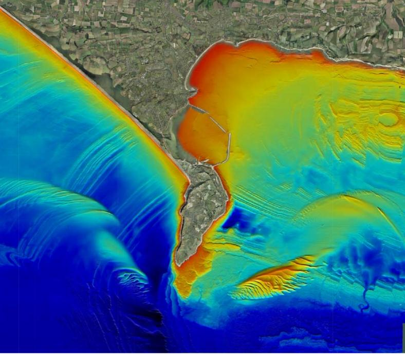
Over 800km² of seabed have been surveyed in great detail to reveal the undersea landscape and over 3,300 photographs and 55 hours of video covering 85km of seabed have been collected and analysed to match seabed communities to the physical features. On the way we have discovered ancient river-channels carved into rock ledges during the last ice-age and been able to link complex geological fault patterns visible in the seabed geology with known structures in the World Heritage "Jurassic Coast".
